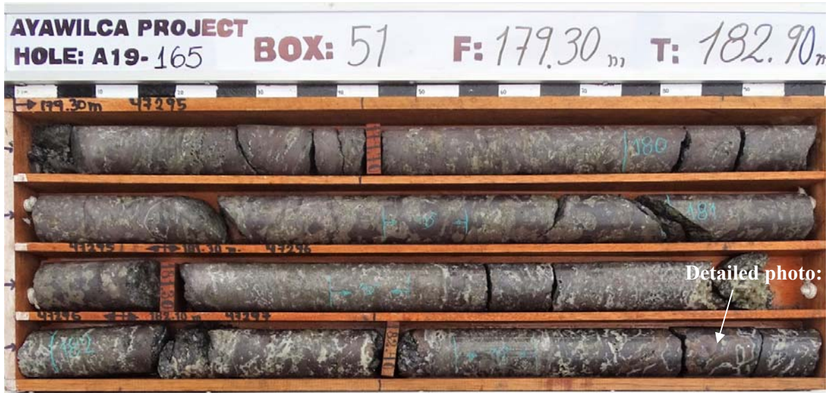
Figure 2. Drill core photographs from the interval in A19-165 grading 18.9% zinc, 42 g/t silver, 0.5% lead, & 584 g/t indium over 7 metres from 178.4 metres. Various phases of zinc sulphides are noted by red-purple-brown hues.
