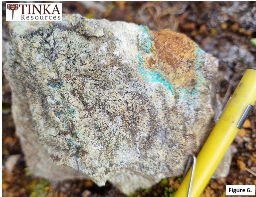
Figure 6 – Photograph of Exoskarn from Area A. Green garnets are pervasive throughout the rock, while copper is observed as turquoise-coloured malachite replacing chalcopyrite
