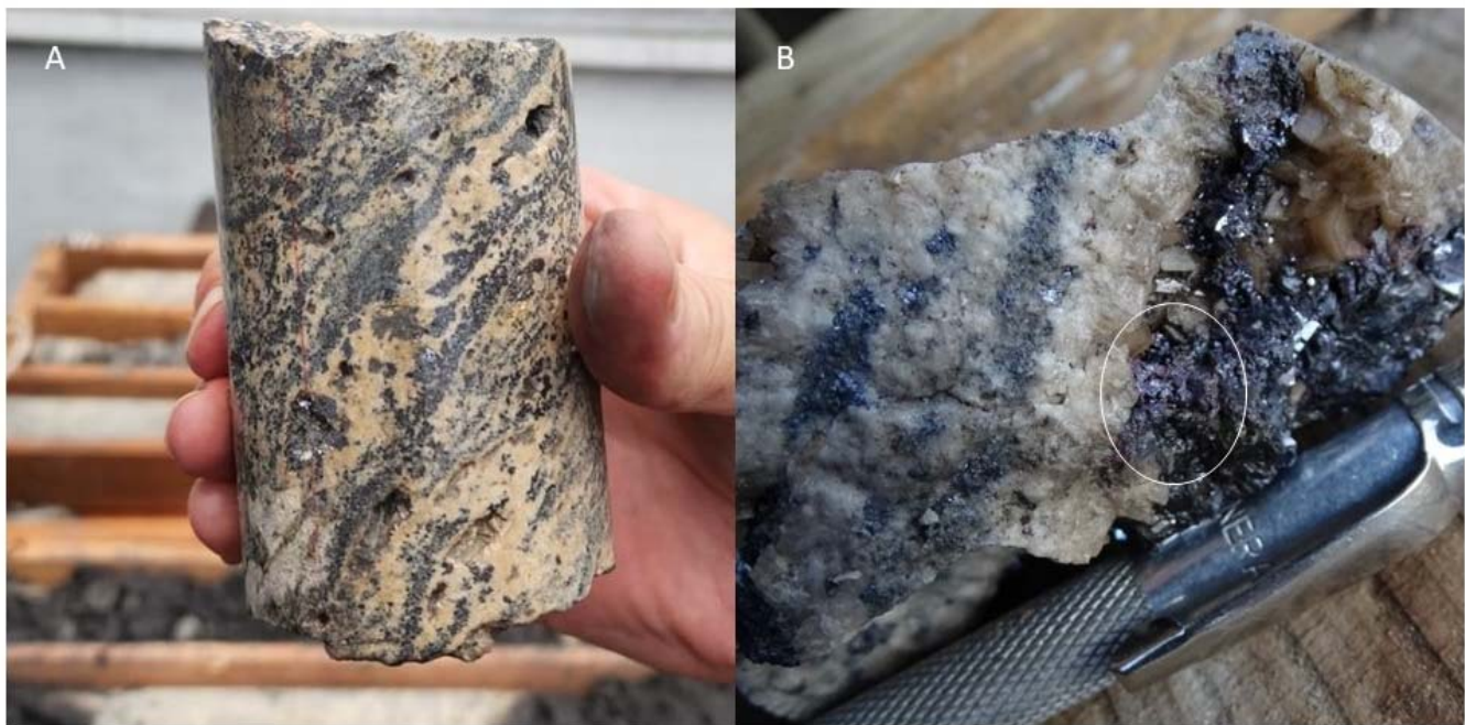
A. Silver Zone (Ag-Pb-Zn Vein) in A23-220 : part of interval grading 2,565 g/t Ag over 0.65 metres. Pyrrargyrite (ruby silver), galena and sphalerite in a banded carbonate matrix.
