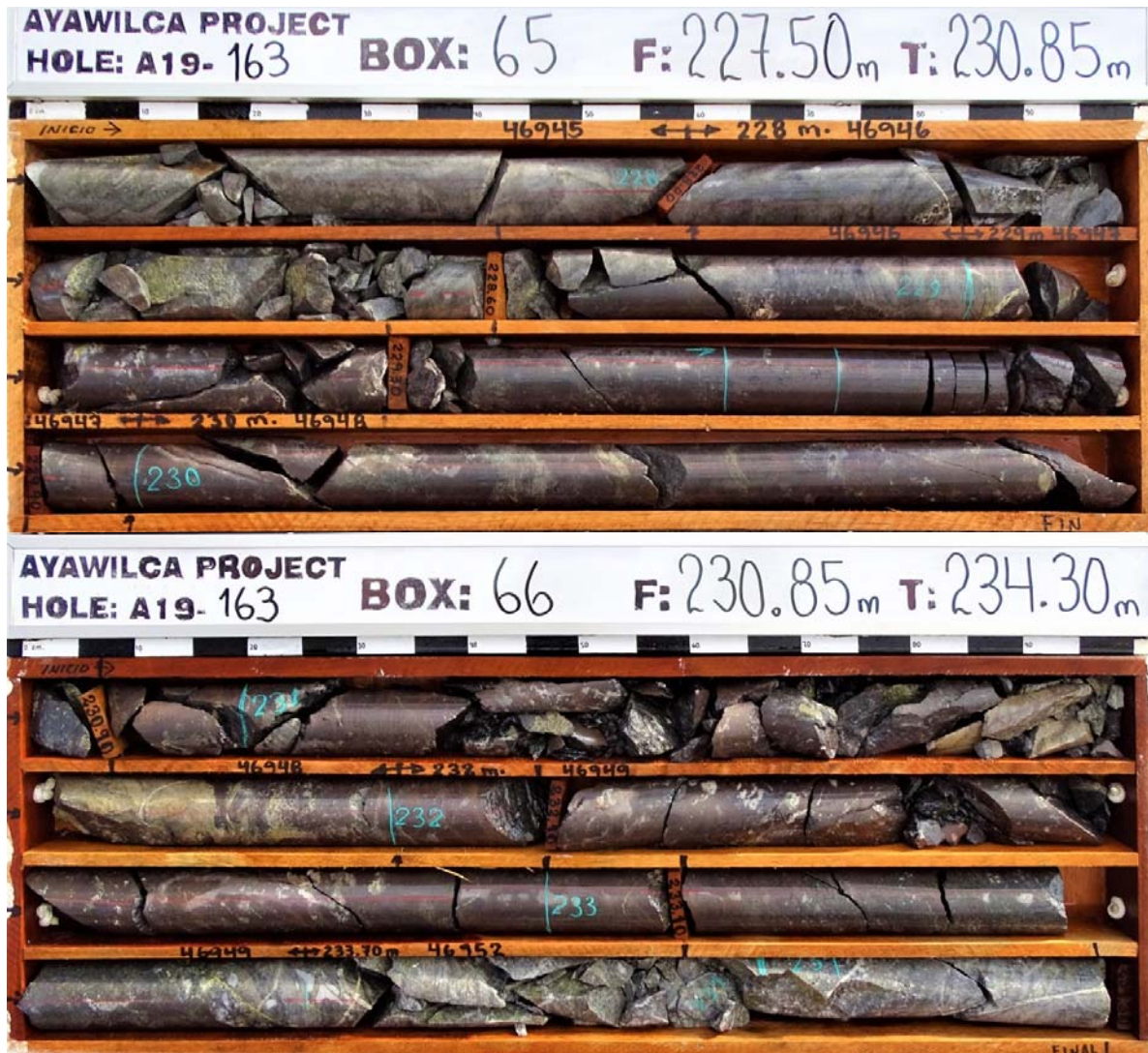
Figure 2. Drill core of high grade interval (228-233.7 m) grading 32.6% zinc, 0.02% lead, 20 g/t silver. Sphalerite is noted by the reddish colour
