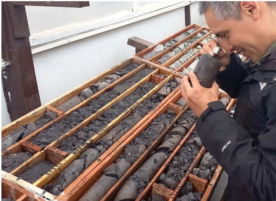
Figure 3. Drill cores from hole A22-202 highlighting the 10.4 metre interval grading 42% zinc
