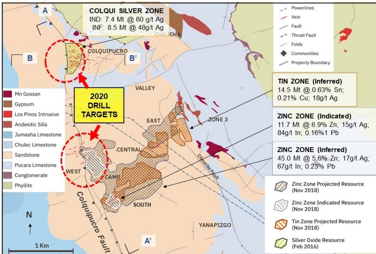
Figure 1. Geology and Mineral Resources of the Ayawilca Project, highlighting 2020 drill targets
