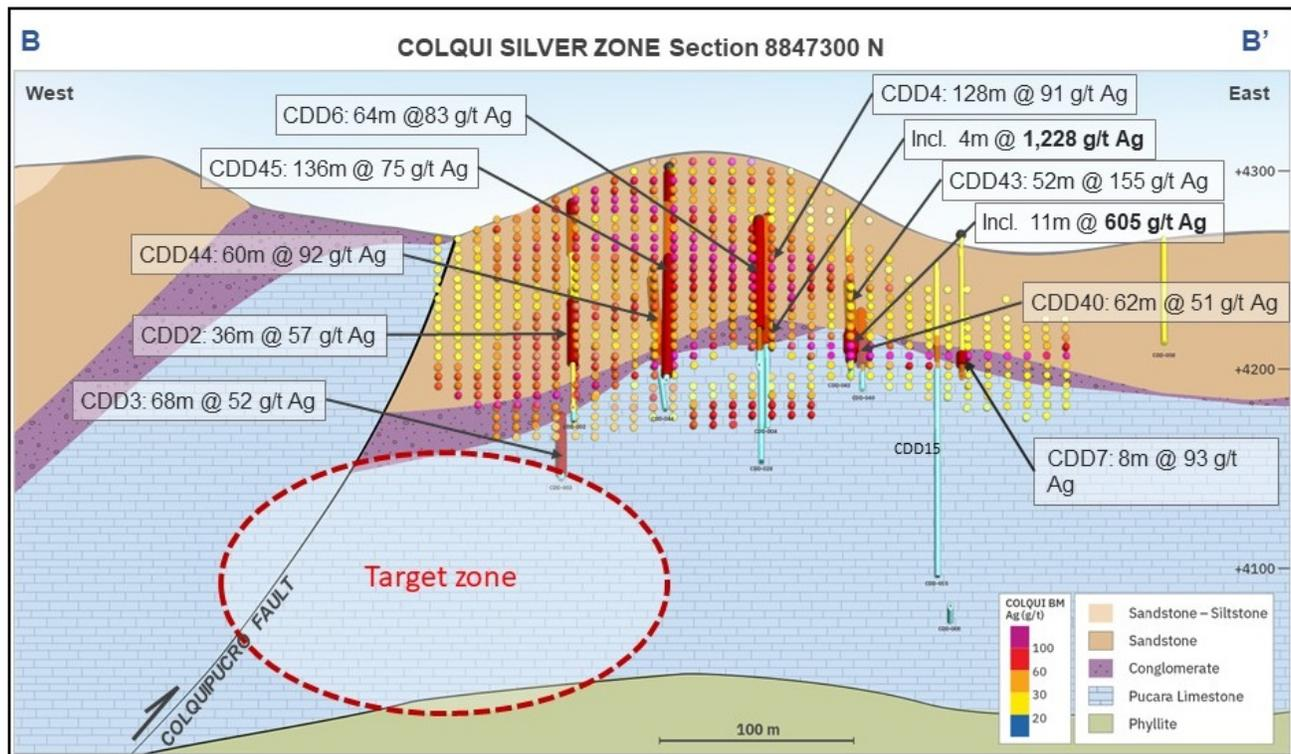
Figure 3. Cross section B-B' (west to east) of the Colqui Silver Zone showing the resource blocks (coloured by grade) and target zone
