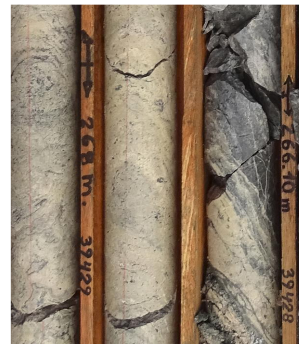
A18-131 Vein textures: carbonates with minor sulphides
